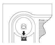
Push down on the Handset retainer until it snaps into place.
